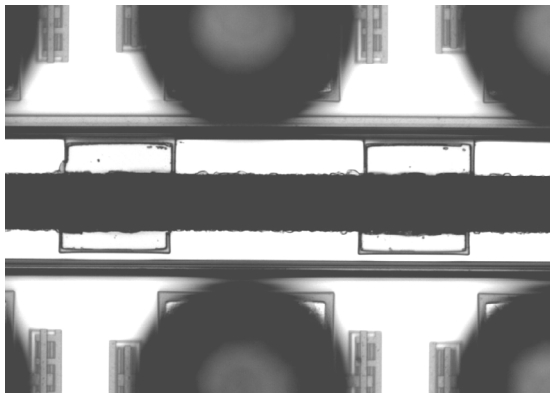
Figure 2. Bumps alongside of dicing street.
